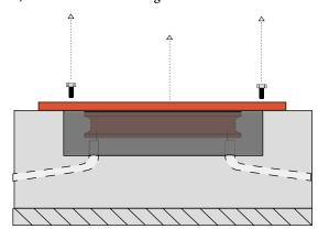
g) Install the RWS scale into the frame and close the manholes
