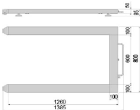
**PWI: Abmessungen in mm**
