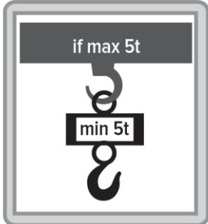
The nominal capacity of the electronic crane scale must not be lower than the maximum capacity of the lifting device.
