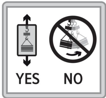
Use the scale EXCLUSIVELY for the lifting and the weighing of suspended loads and for TENSION measurements.
