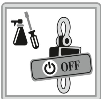
Any maintenance, repair, or cleaning operations must be made with the electronic crane scale turned off.
