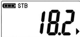
HOLD is hidden. Weight reading is unlocked.
