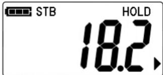
The HOLD indicator on the display turns on, the weight is locked.
